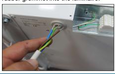
13. Connect the power cable to the terminal block and screw the side cover.
